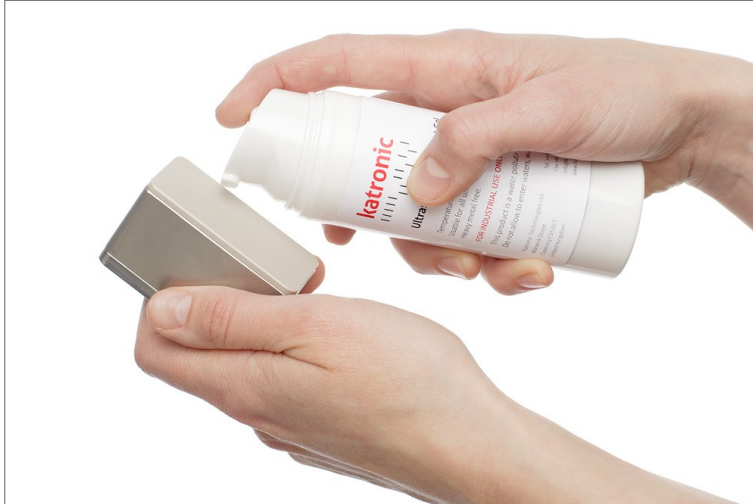
Picture 7: Application of acoustic coupling gel
