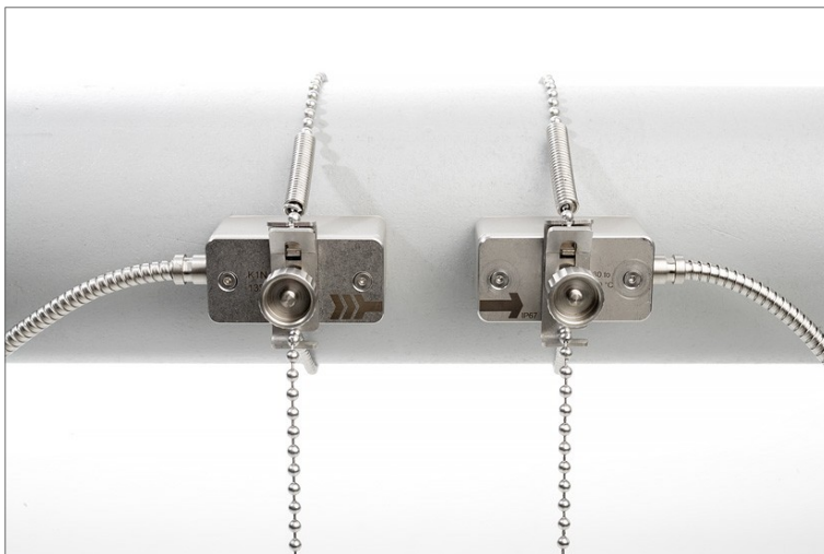
Picture 8: Correct positioning of the sensors
