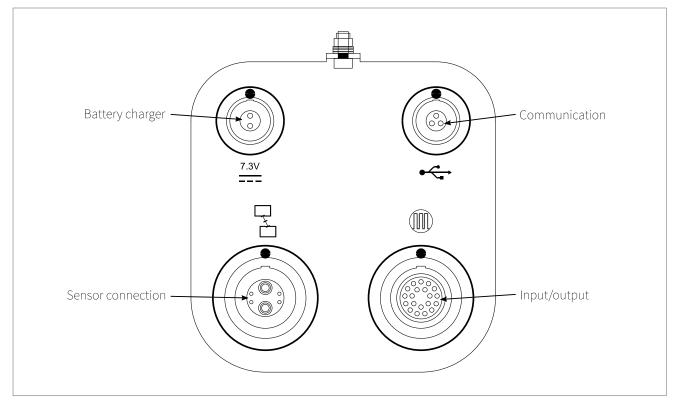
Picture 6: Electrical connection diagram KATflow 210
