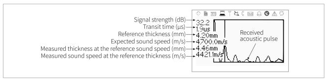
Picture 16: Wall Thickness Gauge (WTG) screen
