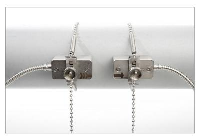
Picture 8: Correct positioning of the sensors
