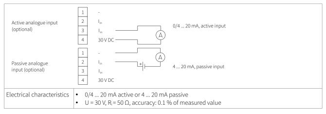
Table 20: Wiring analogue current input 0/4 ... 20 mA
