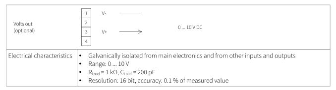
Table 15: Wiring analogue voltage output 0 ... 10 V
