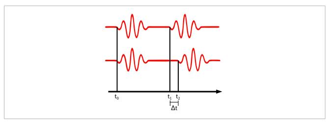
Picture 2: Transit-time measuring principle
