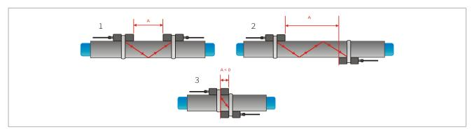
Picture 3: Clamp-on sensor mounting configurations and sensor spacing
