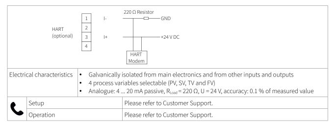
Table 13: Wiring HART® compatible output
