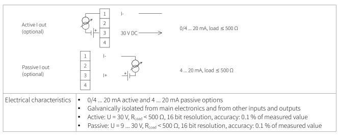
Table 14: Wiring analogue current output 0/4 ... 20 mA
