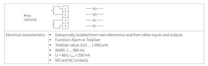
Table 18: Wiring digital relay output
