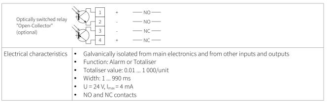
Table 17: Wiring digital open-collector output
