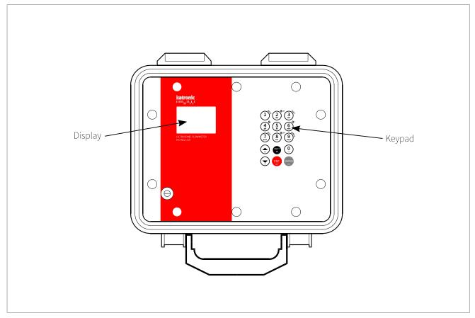
Picture 12: Keypad and display KATflow 210
