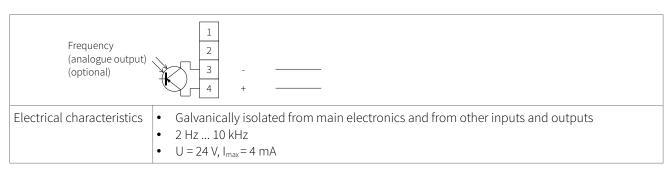
Table 16: Wiring analogue frequency output (passive)
