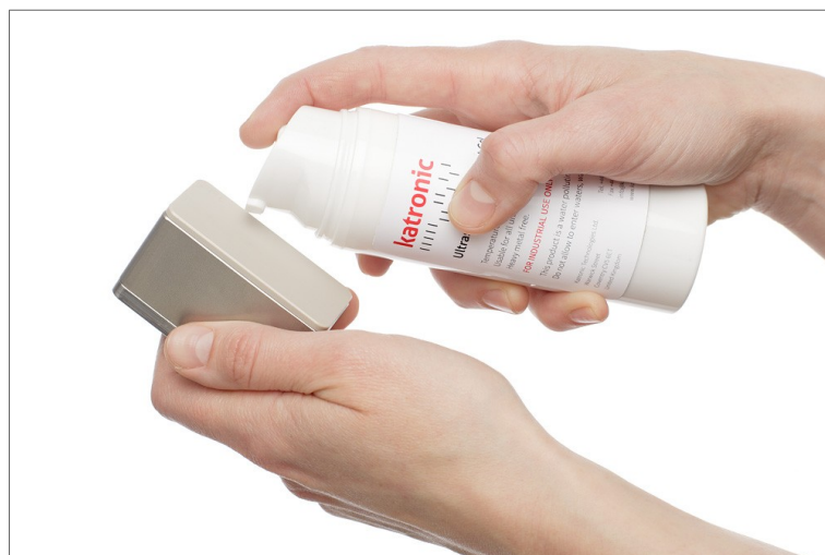
Picture 7: Application of acoustic coupling gel
