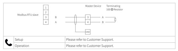
Table 16: Wiring Modbus RTU
