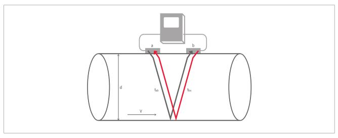
Picture 1: Clamp-on ultrasonic flowmeter configuration
