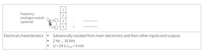
Table 20: Wiring analogue frequency output (passive)
