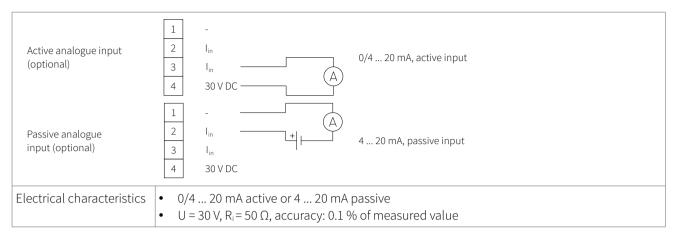
Table 24: Wiring analogue current input 0/4 ... 20 mA
