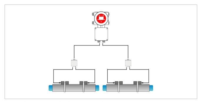
Picture 6: KATflow 170 in a 2-pipe 1-path configuration using optional junction boxes
