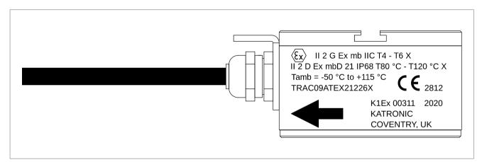
Picture 3: Rating plate sensors K1Ex and K4Ex
