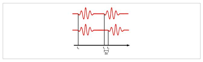
Picture 2: Transit-time measuring principle
