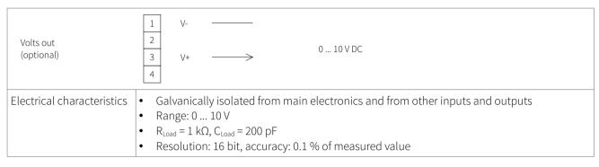
Table 19: Wiring analogue voltage output 0 ... 10 V
