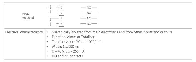
Table 22: Wiring digital relay output
