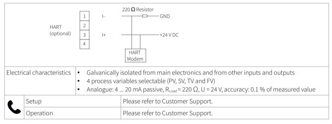
Table 17: Wiring HART® compatible output
