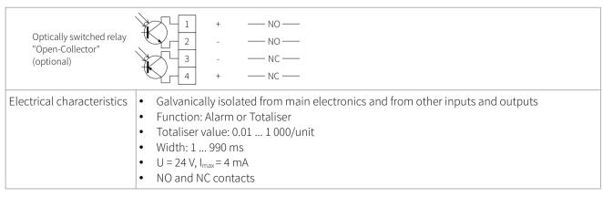
Table 21: Wiring digital open-collector output
