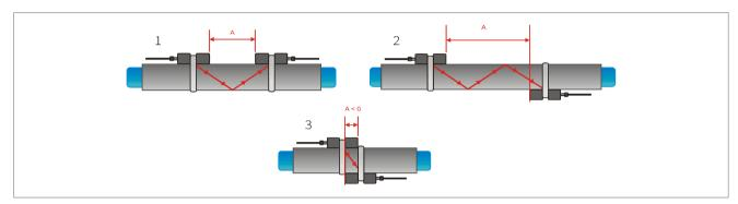
Picture 7: Clamp-on sensor mounting configurations and sensor spacing
