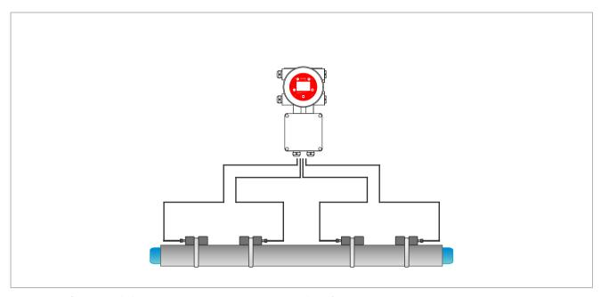
Picture 5: KATflow 170 with direct sensor connection in a 1-pipe 2-path configuration
