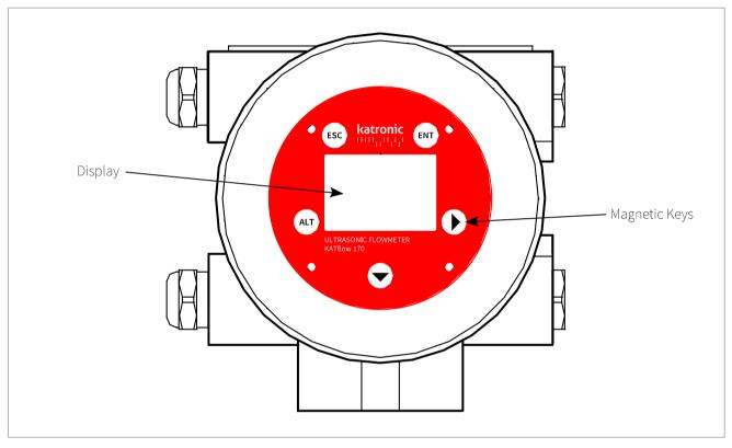
Picture 14: Keypad and display KATflow 170
