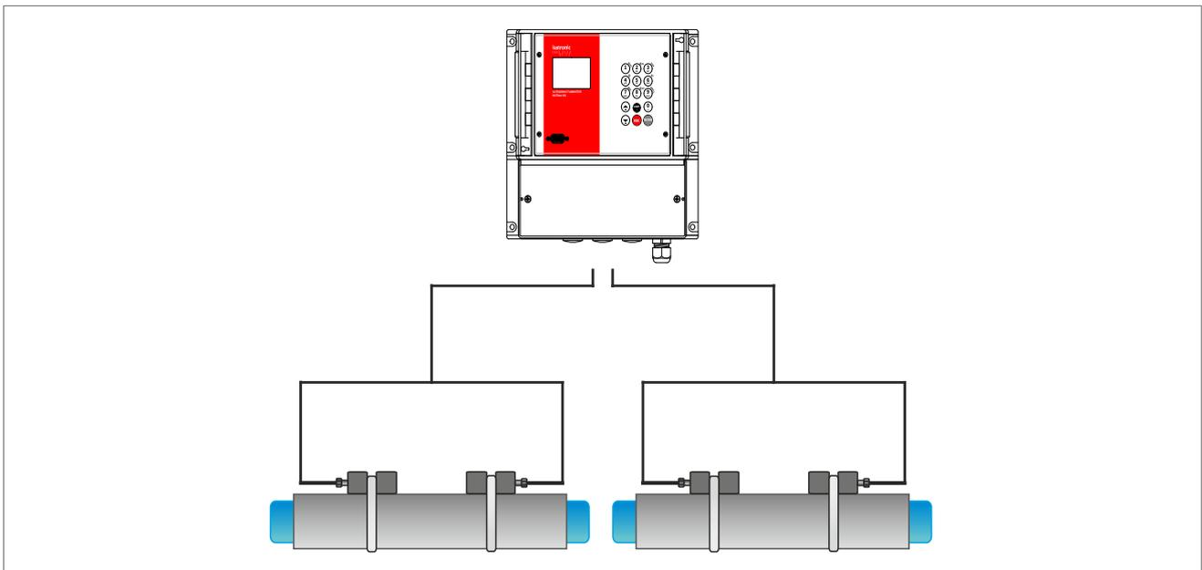
Picture 4: KATflow 150 in a 2-pipe 1-path configuration
