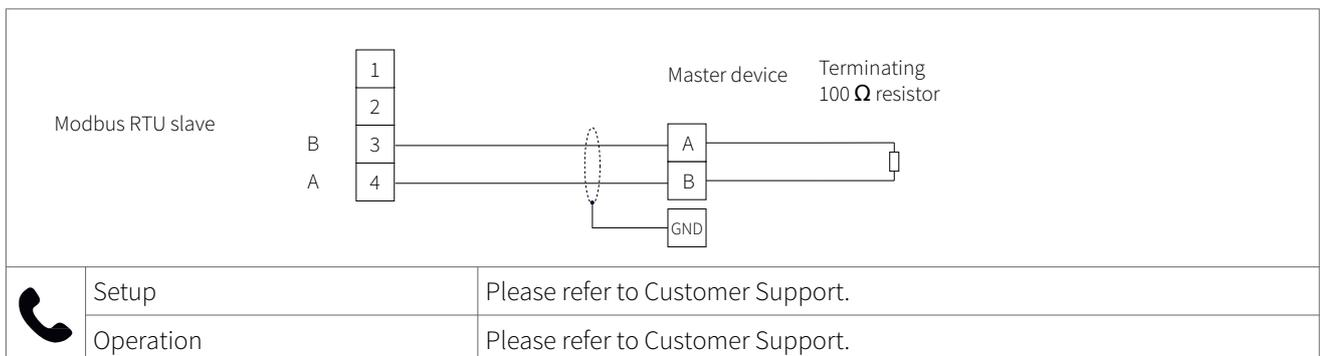
Table 18: Wiring Modbus RTU
