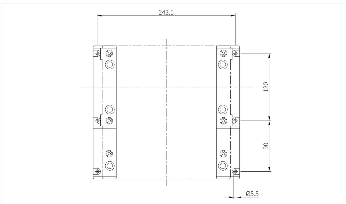
Picture 7: Drilling aid for wall mounting KATflow 150
