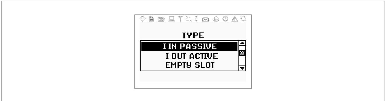
Picture 14: Display example passive current input slot 1, active current output slot 2
