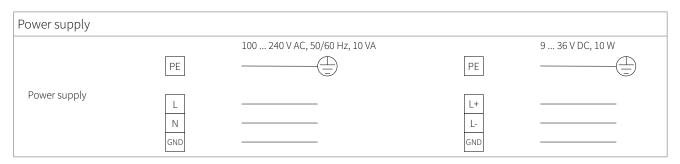
Table 3: Electrical diagram power supply for the KATflow 150 flowmeter
