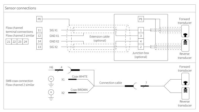
Table 4: Electrical diagram sensor connections for the KATflow 150 flowmeter
