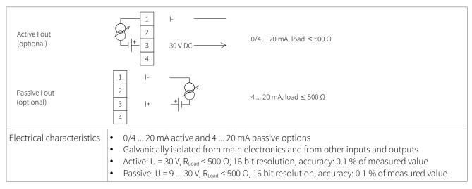
Table 20: Wiring analogue current output 0/4 ... 20 mA
