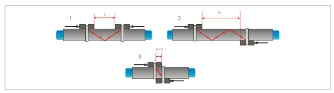
Picture 5: Clamp-on sensor mounting configurations and sensor spacing
