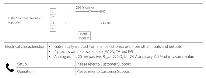
Table 19: Wiring HART® compatible output
