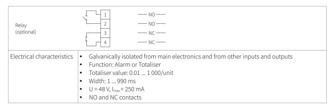
Table 24: Wiring digital relay output
