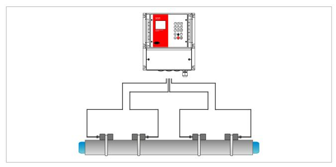
Picture 3: KATflow 150 with direct sensor connection in a 1-pipe 2-path configuration
