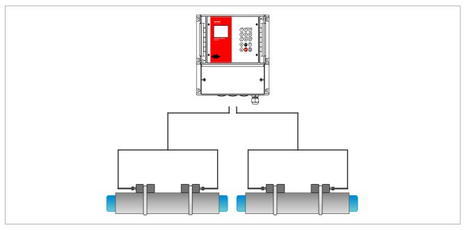
Picture 4: KATflow 150 in a 2-pipe 1-path configuration
