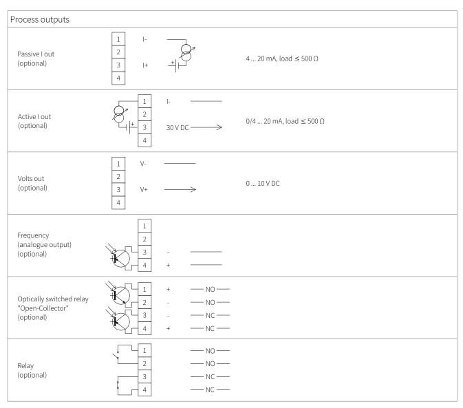
Table 5: Electrical diagram process outputs for the KATflow 150 flowmeter
