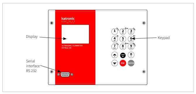
Picture 12: Keypad and display KATflow 150
