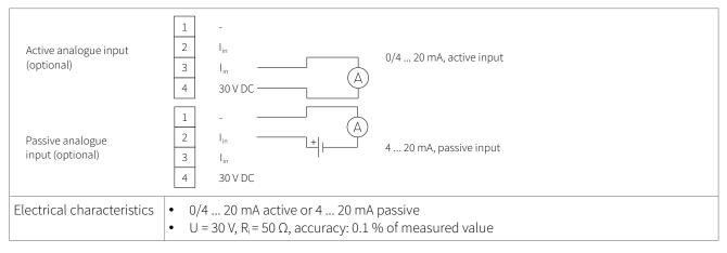
Table 26: Wiring analogue current input 0/4 ... 20 mA
