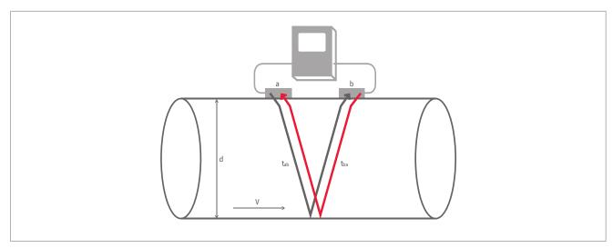
Picture 1: Clamp-on ultrasonic flowmeter configuration
