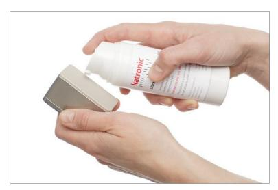
Picture 8: Application of acoustic coupling gel
