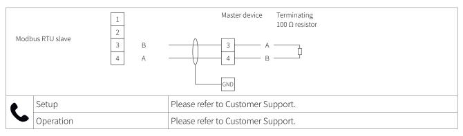
Table 18: Wiring Modbus RTU
