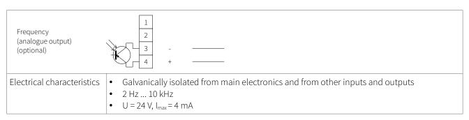
Table 22: Wiring analogue frequency output (passive)
