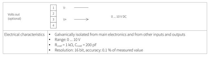
Table 21: Wiring analogue voltage output 0 ... 10 V
