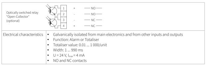
Table 23: Wiring digital open-collector output
