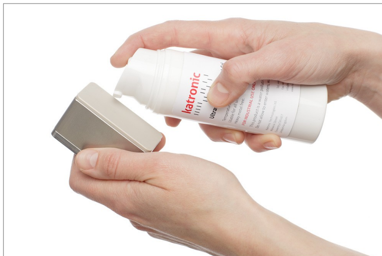
Picture 7: Application of acoustic coupling gel
