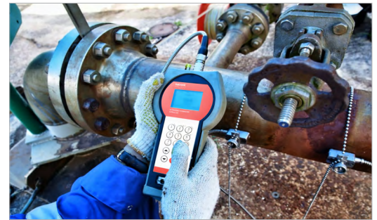
Supra Indodrill used a clamp-on KATflow 200 for measurement of debit from water wells in Indonesia.
