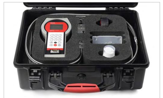
The KATflow 200 offers mobility, ease of installation and operation.
