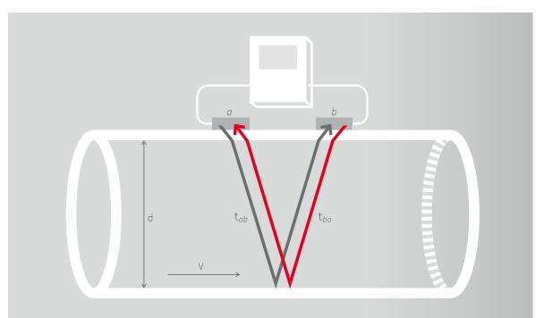
Sensors *a* and *b* work alternately to send and receive ultrasonic pulses. The sound waves *ab* travelling with the flow move faster than those travelling against it *ba*.
